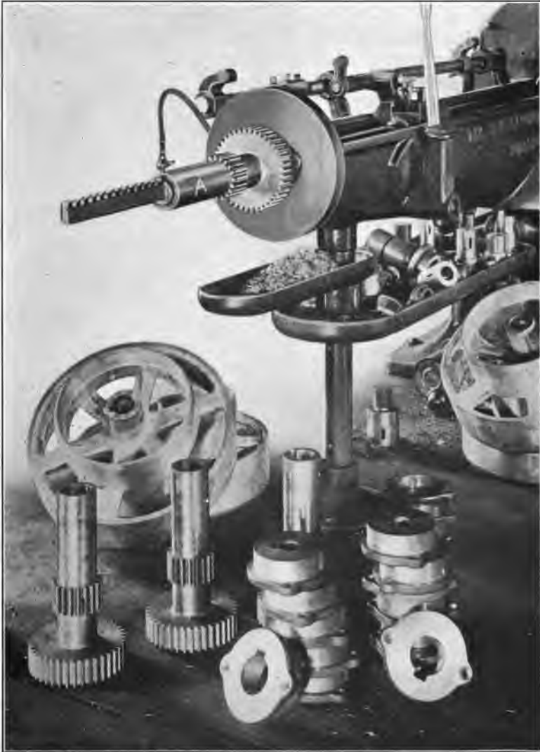
FIG. 21.—Machine set up for broaching keyways.
